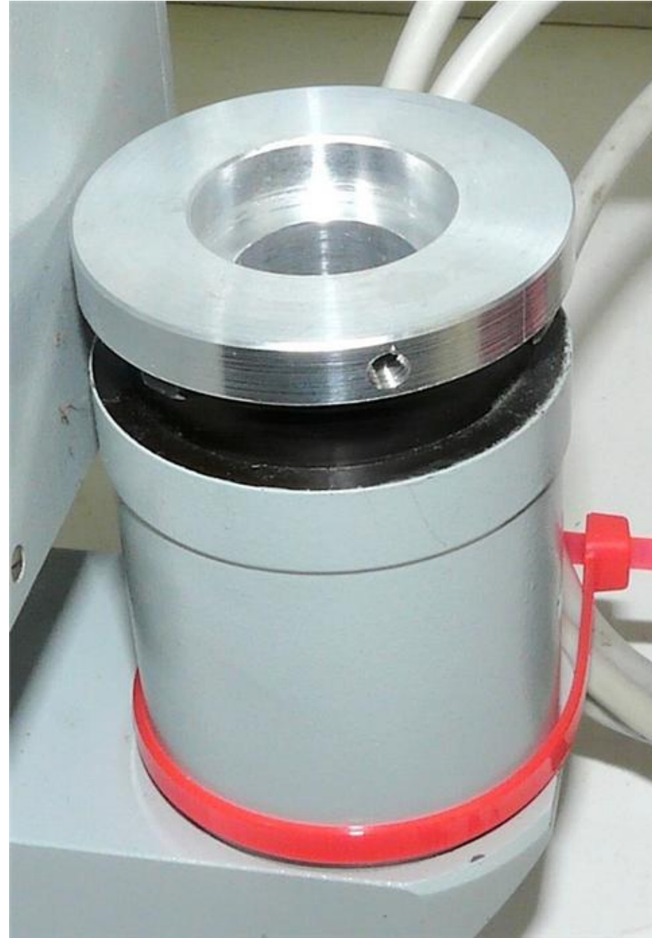
(2) Nanodyne adapter installed in lamp housing. A ball plunger provides friction to keep it in place.
