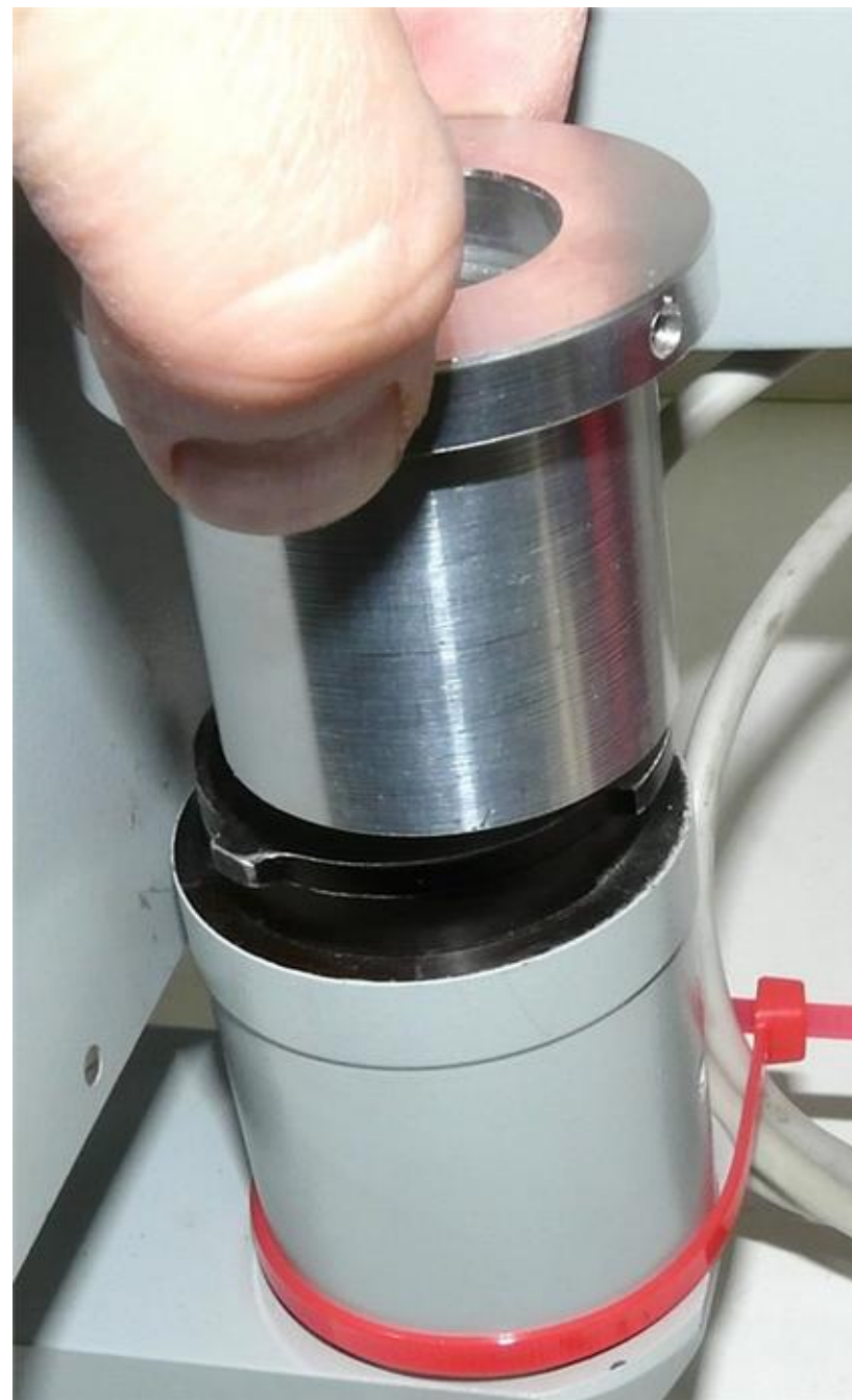
(1) Insert the Nanodyne adapter into the lamp housing.
