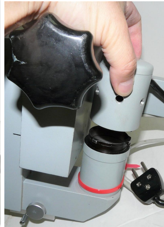
(2) Twist and remove cover.
