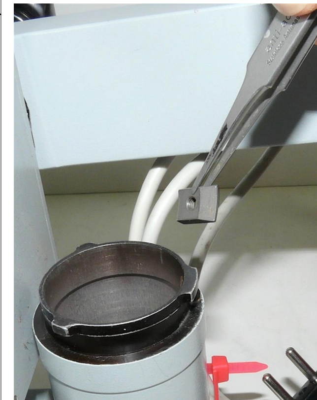
(5) Remove the nut the screw was in.
