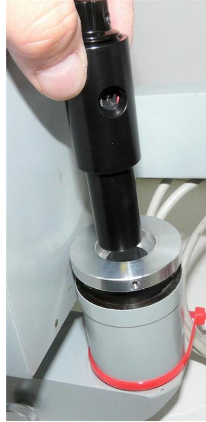
(3) Insert the Nanodyne illuminator into the adapter.
