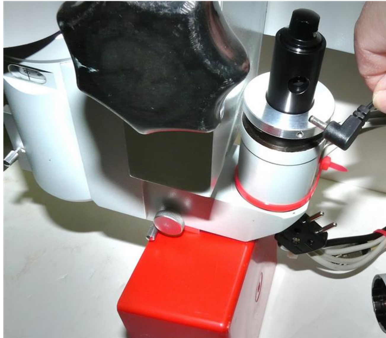
(1) Set up the microscope so it is focused on a flat surface. Plug the USB end of the power cord into the power supply. Plug the other end into the illuminator. Plug the power supply into an AC outlet.
