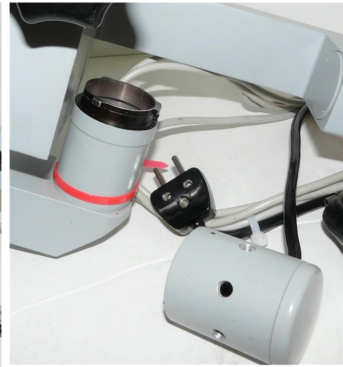
(3) Lamphouse cover removed.
